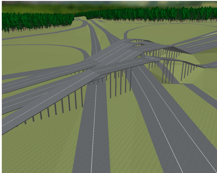
Figure 4.10.: Bridges at a motorway junction, exposing the shortcomings of our objective function. There is no incentive to smooth the bridge surface, and ground level roads are kept close to the approximated terrain at all costs.
